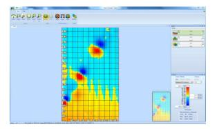
Compensation of single probes from a multi-probe system
