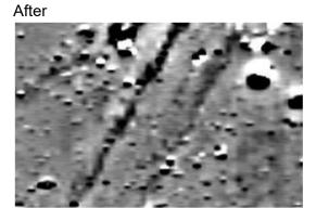
Removes stripes that occur parallel to the moving direction.
